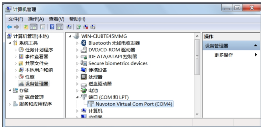
Figure 1: The port hardware tips of Nuvoton Virtual Com prot(comx) after the driver is installed succedssfully.
